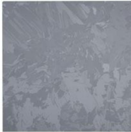
Solar Multicrystalline Wafer: 156mm x 156mm
